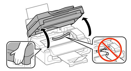
**Caution:** Do not touch the flat white cable inside the printer. Do not lift the scanner unit while the document cover is open.
